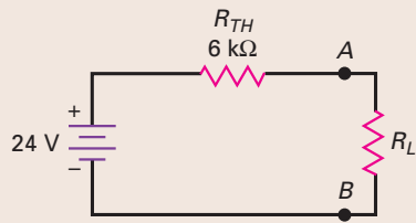
Figure 1-10 Thevenin circuit for Fig. 1-9a.
