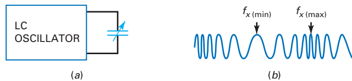
Figure 21-48 (a) Variable capacitance changes resonant frequency of LC oscillator; (b) sine wave has been frequency-modulated.
